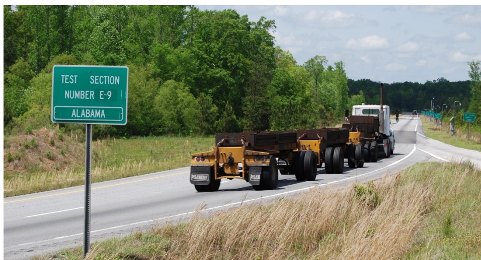
FIGURE 7 Heavily loaded triple-trailer used for accelerated loading on the Test Track.
