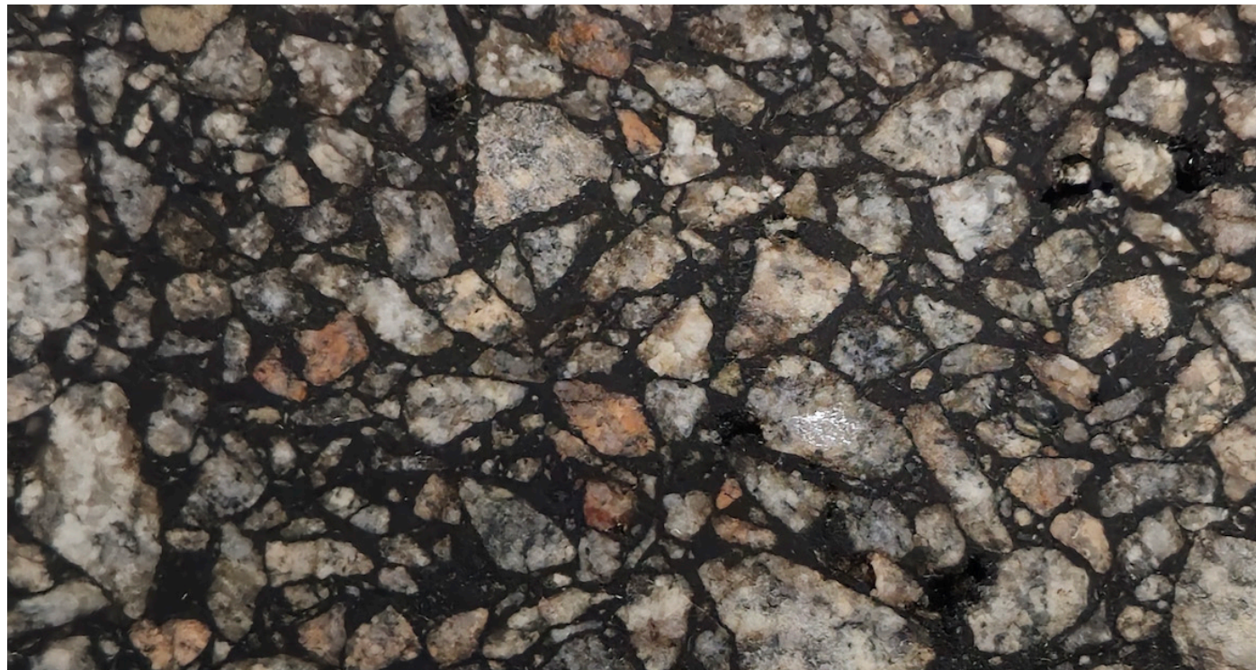
Figure 7. Close-up of aggregate skeleton of an SMA mix.
