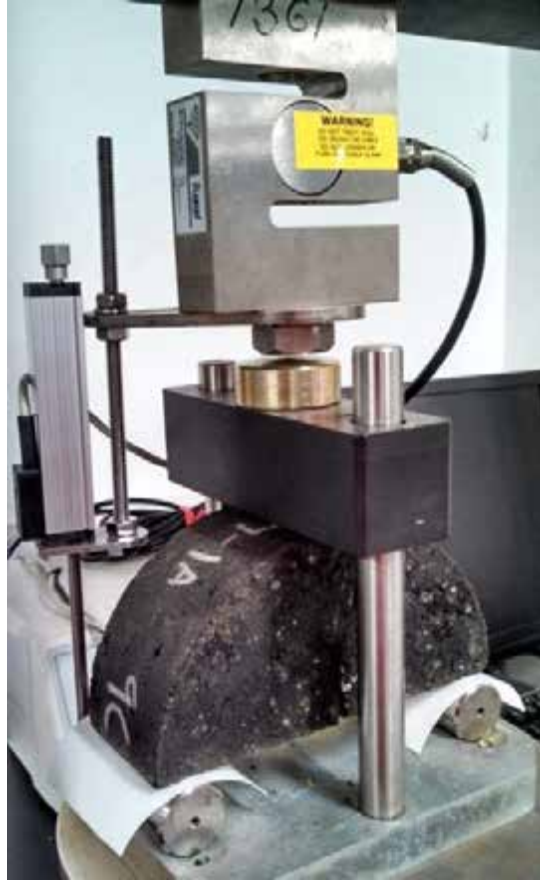
Figure 6 Semi-Circular Bend Test
