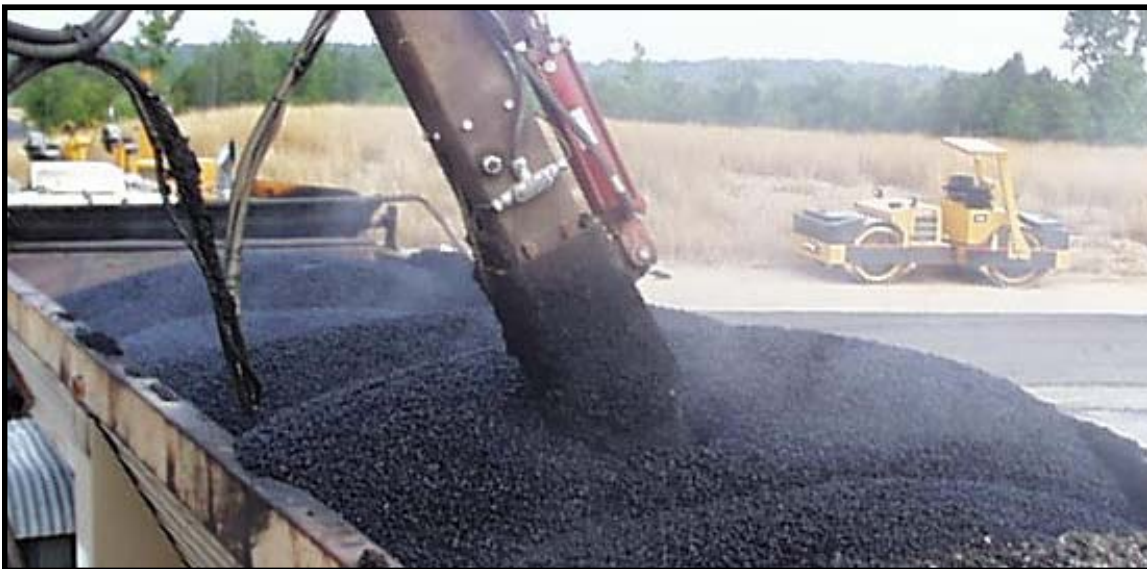
Figure 4. Sampling Mix at Plant with Automated Robotic Sampler
