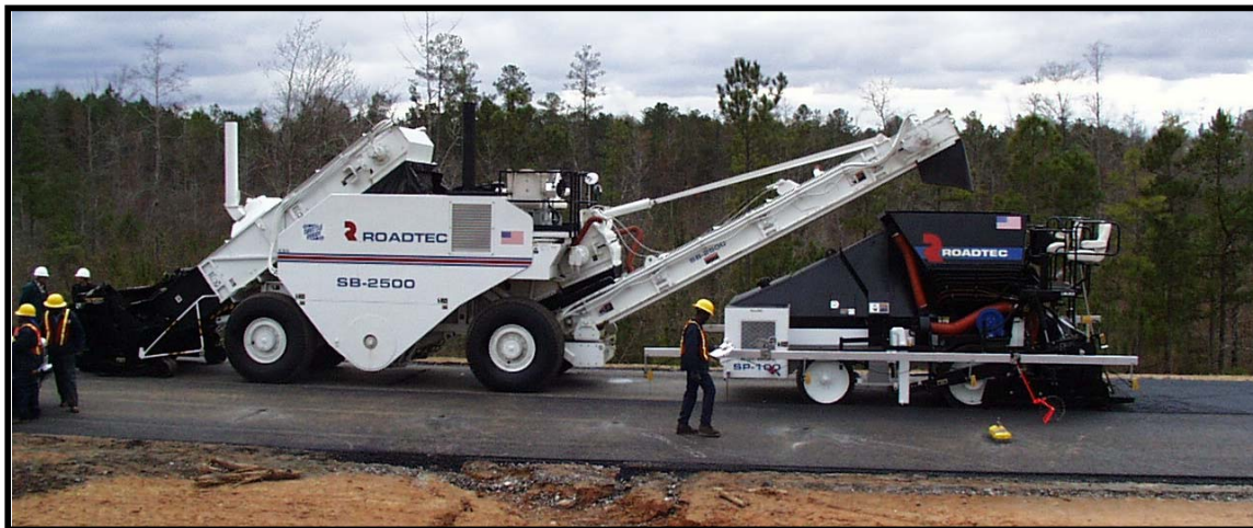
Figure 7. Gravity Feed Paver Used to Place Experimental Mixes
