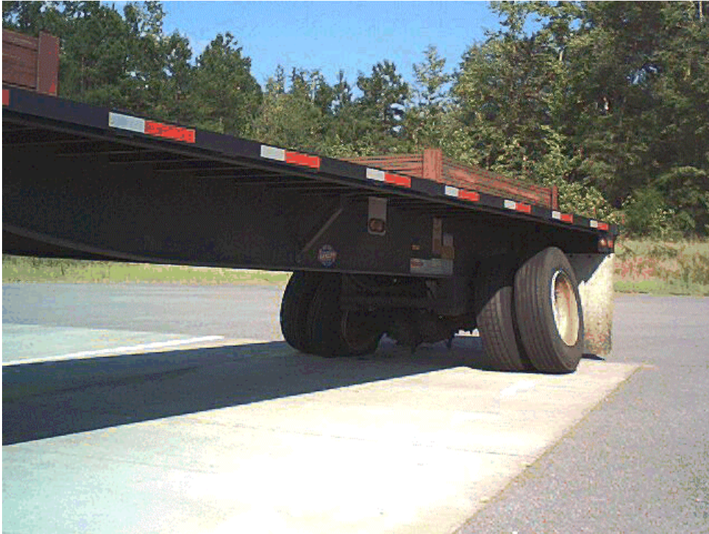
Figure 15. Broken Rear Axle in Last Trailer of Train
