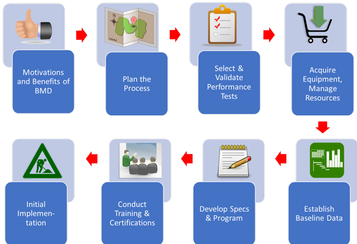
Figure 1.3. Illustration of the Major Steps in the Process of Implementing Performance Specifications.
