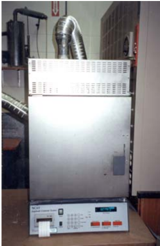
NCAT ignition oven from Barnstead Thermolyne (1995).
