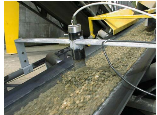
Microwave aggregate moisture probe installed on a conveyor belt was demonstrated in the QC open house (July 2004).
