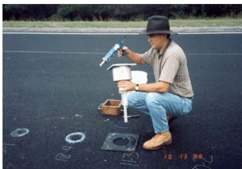
Allen Cooley with NCAT permeability device (1998).
